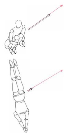
STRAIGHTENING OUT OF A TUCK will cause the angular velocity (*black arrow*) of a diver to decrease fivefold because his moment of inertia is five times larger in the straight position than in the tucked one. The angular velocity and moment of inertia can vary inversely as long as their product, the angular momentum (*colored arrow*), remains constant.
